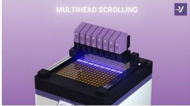
Below we have created an example of the throughput that can be achieved, where a 30 x 30 x 30 cube is produced by scrolling light engines with different configurations (2, 4, and 8 light engines) compared to a traditional static DLP machine with 2, 4, and 8 static heads. The example also takes into account a "high energy" resin and a "standard" resin.
