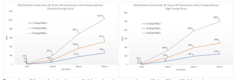
Examples of throughput using our light engines in comparison with traditional light engines.
