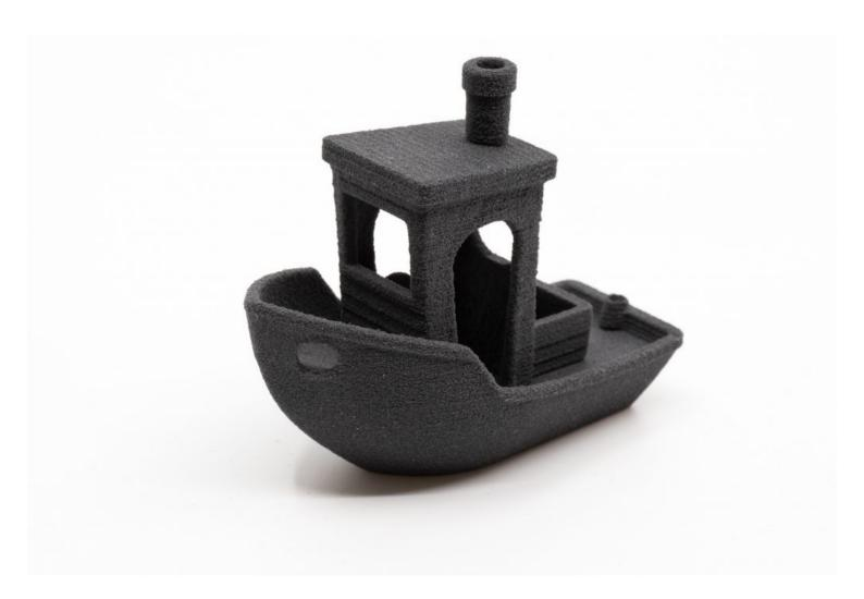
Using their own DLP-based, powerful IR light engine instead of the traditional single focused laser beam, known from SLS technology, core benefits such as drastically increased print speed, resolution, and build area are the result. Visitech aimed to remove the limitations of the widely used Selective Laser Sintering (SLS) method and develop powder bed fusion (PBF) as a better candidate for industrial applications. This would require high throughput and resolution.
